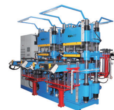
KIIWOO INDUSTRY 全自动平板硫化机(热水袋专用成型机设备) Automatic flat plate vulcanizing machine (special molding machine for hot water bag)
